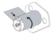
**13.** Reinstall the hook. Insert the short end of the hook into the hole in the center of the adjusting nut (1). Insert the long end of the hook into the small hole on the guide plate (2).
